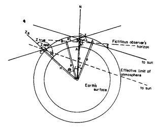
FIGURE 4-3.—Geometry employed in computation of refraction.
