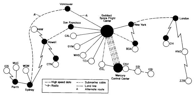
FIGURE 2-8.—Data circuits for Project Mercury.
