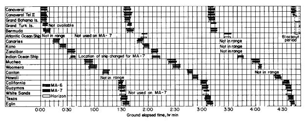
FIGURE 2-15.—Comparison of telemetry coverage times for MA-6 and MA-7.
