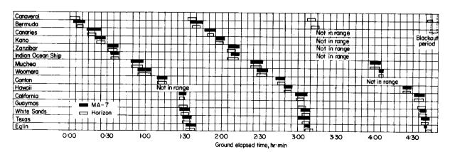
FIGURE 2-6.—Acquisition system coverage.
