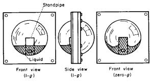
FIGURE 1-13.-Zero-gravity experiment.
