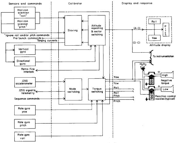
FIGURE 1-5.—Control system schematic diagram.
