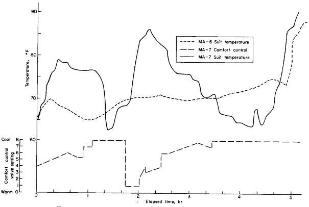
FIGURE 1-11.-Suit-inlet temperature and comfort control valve setting.
