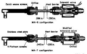
FIGURE 1-4.---Comparison between MA-6 and MA-7 thrusters.
