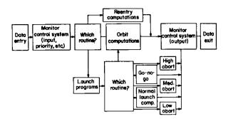
FIGURE 2-10.-Real-time monitor control system.
