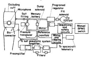
FIGURE 1-8.—Semiautomatic blood-pressure measuring system.
