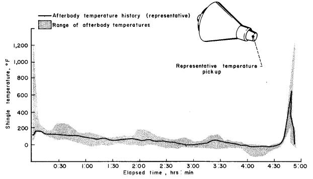
FIGURE 1-3.—Afterbody temperature from low-level commutator circuit.
