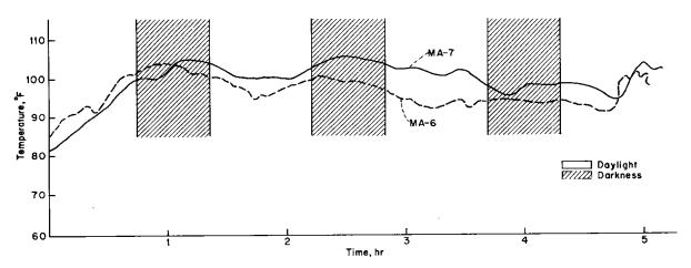
FIGURE 1-10.—Cabin-air temperatures.
