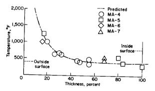
FIGURE 1-2.-Maximum ablation-shield temperatures.
