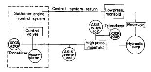
FIGURE 1-14.-Launch-vehicle hydraulic diagram.
