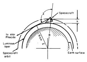
FIGURE 4-1.--Parameters used to calculate height of layer.
