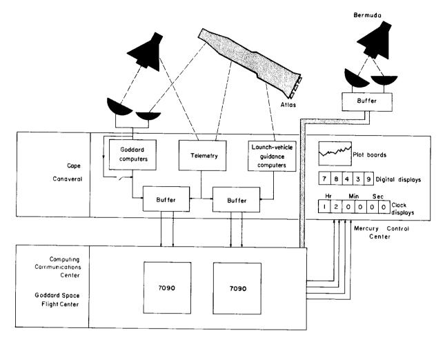
FIGURE 2-11.—Computer data sources during launch.
