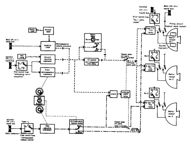
FIGURE 1-12.-Retrosequence schematic diagram.
