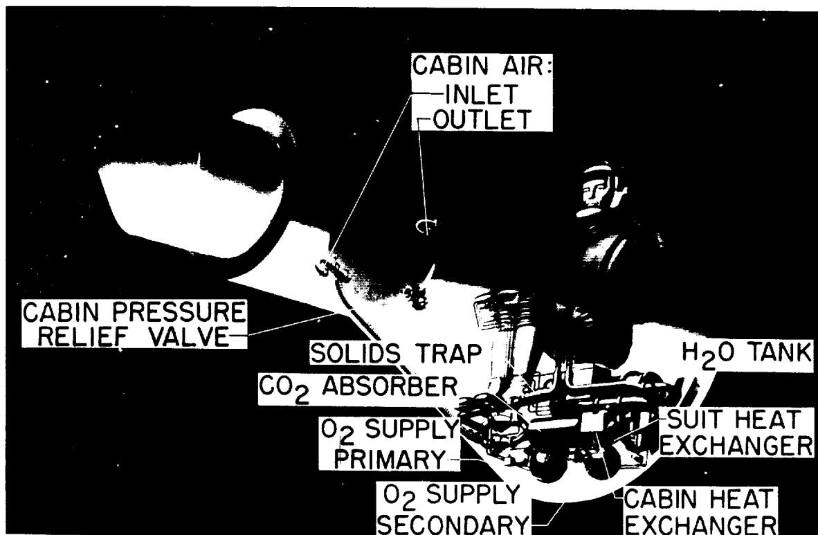
FIGURE 2-19.—Approximate physical arrangement of spacecraft environmental control system.
