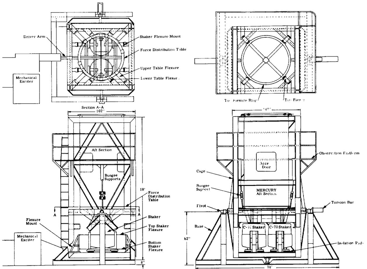
Figure 6-3. Vertical Test Fixtures
