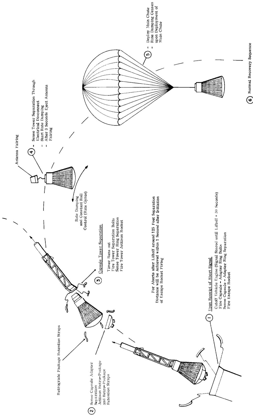
Figure 5-6. Abort After Liftoff up to Normal Engine Cutoff
