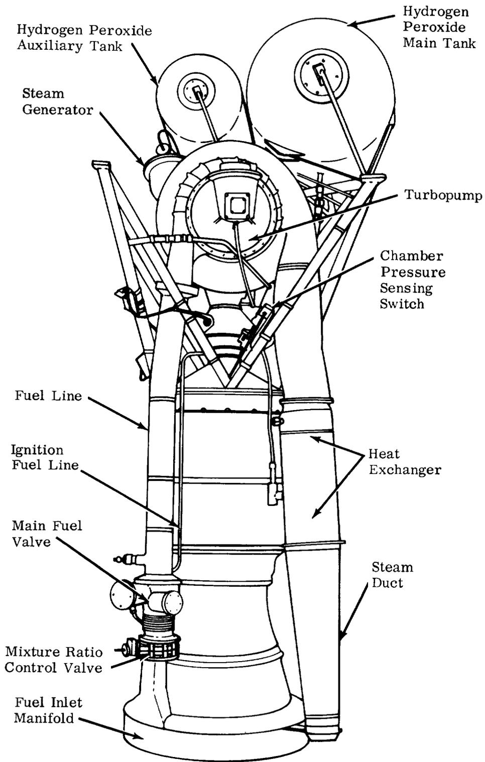
Figure 4-3. A-7 Rocket Engine
