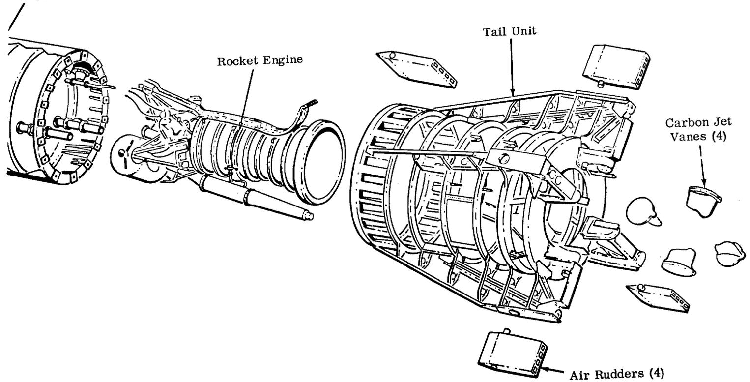
Skin thickness was 0.090 inch on the aft unit, 0.063 inch on the fuel tank, 0.080 inch on the LOX tank, and 0.125 inch on the tail unit. Glass wool was used to insulate the LOX tank bulkheads and the fuel feed line, which passed through the LOX tank.
