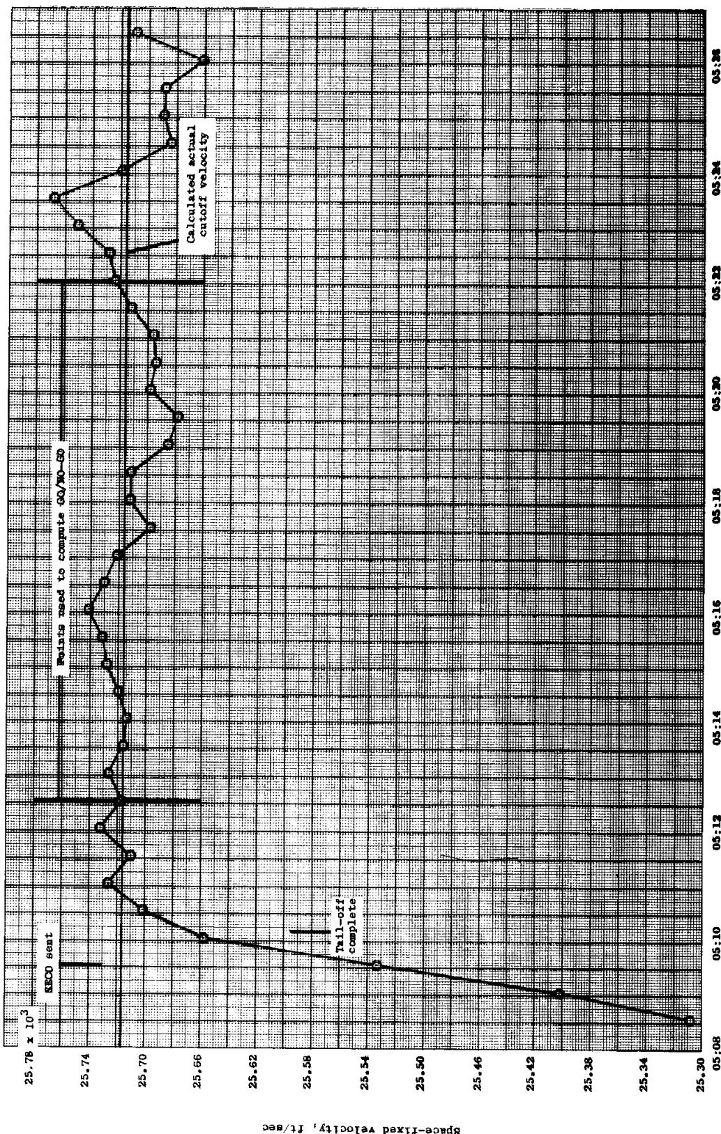
Figure 4.3-1. - Space-fixed velocity and flight-path angle in the region of cutoff using General Electric - Burroughs data.
