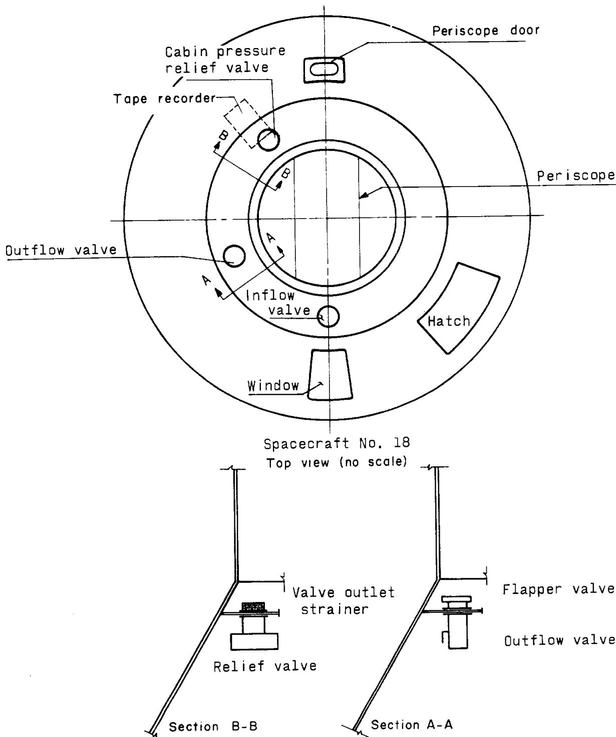
Figure 5.5.7-1.- Sketch showing location of valves in spacecraft small pressure bulkhead.
