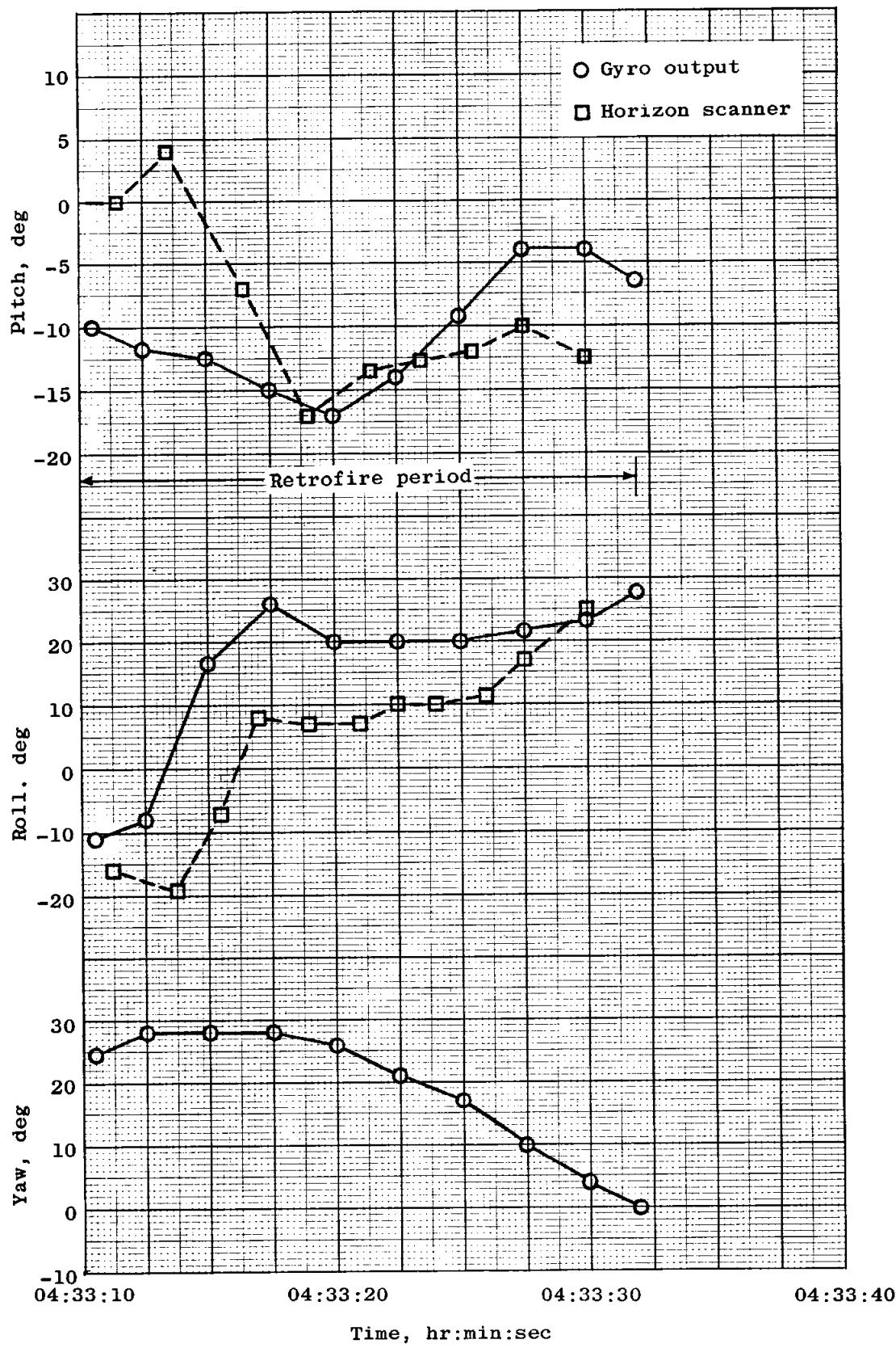
Figure 7.2.3.6-1-- Horizon scanner and gyro output during retrofire period for MA-7.
