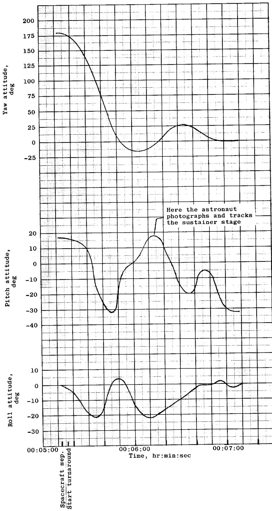
Figure 7.2.3.1-1. - Turnaround maneuver; fly-by-wire control mode, rate and attitude gyro indicator.
