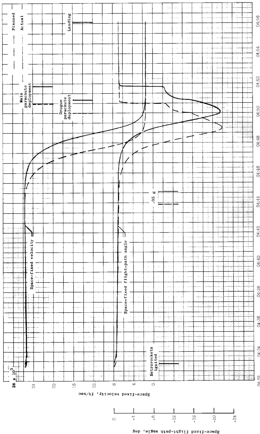
(b) Space-fixed velocity and flight-path angle.
