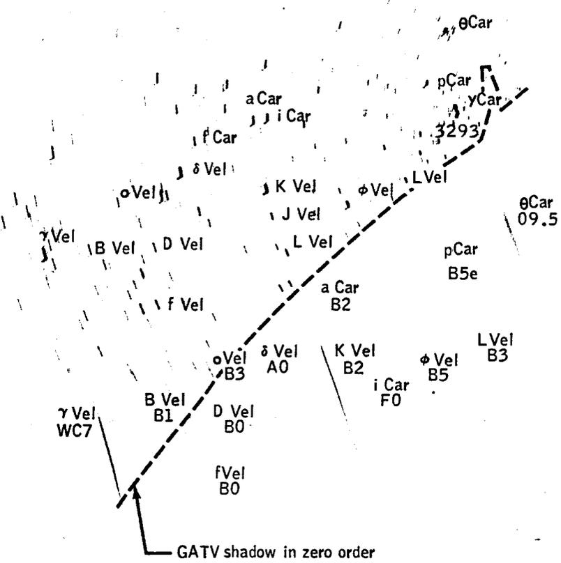
These spectra were obtained during standup EVA with the general purpose 70-mm camera, taken at an f setting of 3.3 using a 73-mm lens and an objective grating. The spectra extend from 2200 Å to about 3500 Å. The spacecraft was docked with the Gemini X GATV resulting in an apparent field rotation due to orbital motion of 80 arc seconds during the 20-second exposure period.
