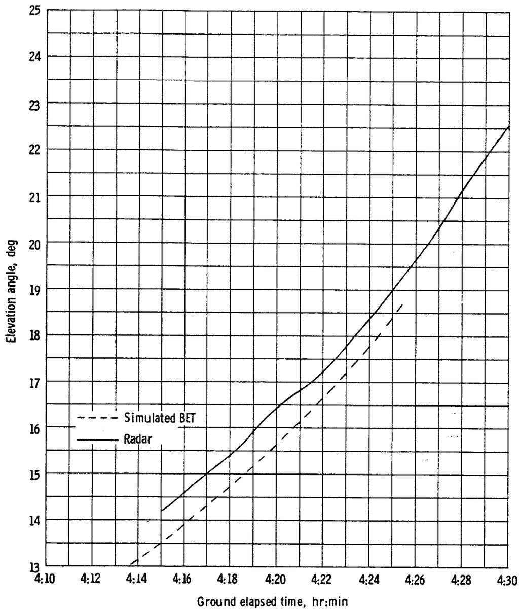
Figure 5.1.5-10. - Comparison of spacecraft radar-measured elevation angles with postflight-simulated angles.
