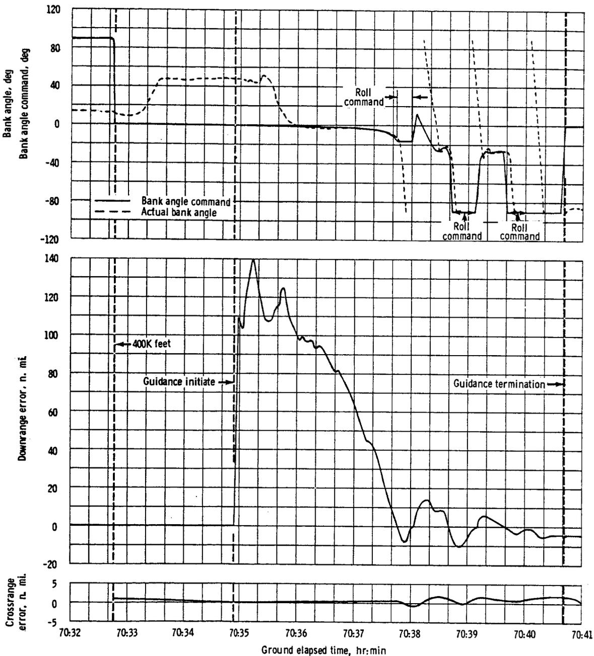
Figure 5.1.5-24. - Reentry guidance parameters.
