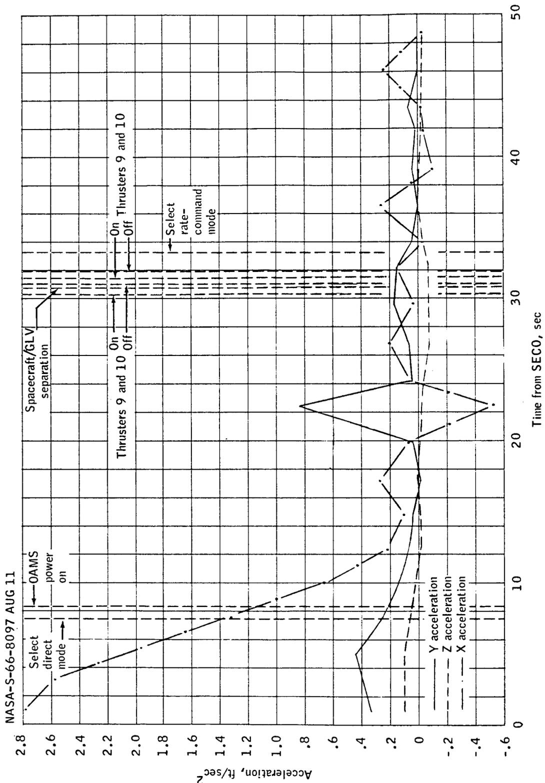
Figure 5.1.5-2. - Spacecraft acceleration measured after SECO.
